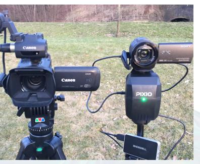
include auto-follow cameras from companies such as Move 'N See and SoloShot that automatically track each player for close-ups. For analysis using even more angles, live 'slave' computers can be synchronized with the main system, with each secondary system supporting four more cameras with Magewell converters.
